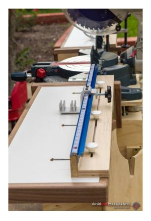
The fence is simply 2 pieces of wood joined with a glued & screwed butt joint. I mounted my fence using a wooden slot with adjustable knobs which slide in T-track. This lets me adjust it if I get a different saw and it lets me adjust the width of the fence. I can slide the fences away from the saw if I need to cut something extra long.
